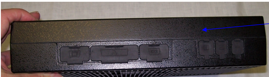
Sealed Rubber plugs and gaskets to keep out the water
