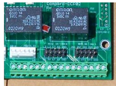
Digital I/O and 2) 5A Dry Contact Relays 4 Analog inputs for general purpose
