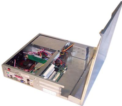
The new 7596 product provide an outstanding combination of price, unmatched performance, and versatility. Whether used as a single, stand-alone system or in a LAN environment, these systems deliver the speed and solid functionality needed for off-the-shelf or customized applications. The 7596 offers Pentium 4 processor, 2GB DDR 266 memory, fast ATA133 hard disk drive access, and Intel 64M AGP 3D graphics. Integrated Ethernet , video, and Stereo Sound.
